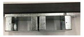
Mount one or two boxes to second bracket as necessary using 10-32X3/16 THMS and box to box connector.
