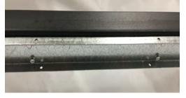
Mount first half of bracket to the frame using 4 #8X1/2" hex head screws. <u>If these are on the lower bar it is important to mount these before the frames are stood.</u> Bracket should be aligned offset from the pair of power openings.
