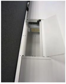
Bracket mounts to rear cross bar in desired location using 6 #8 X ½ dp screws. For use with access flap installation. Using single sided(blank one opening), one left and/or one right with the center of the access area open for user is recommended. Wire in accordance with local electrical codes.
